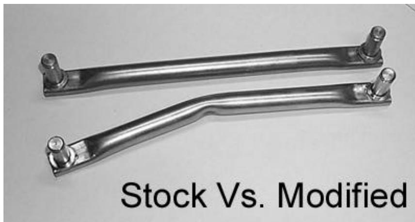
The newly modified lever now has the proper clearance for the Ultimate Short Shifter.
