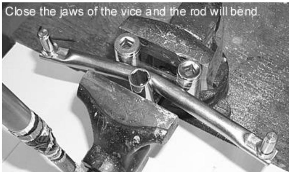
Slowly close the jaws of the vice and the selector rod will bend with a nice smooth radius of the socket. Be sure that the "pins" of the selector rod are pointed straight up so that it bends straight.
